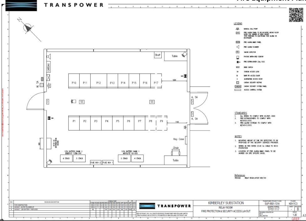
Sleeve Three – Fire Equipment Plan
